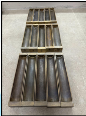
15 units of Linear Shrinkage mould
